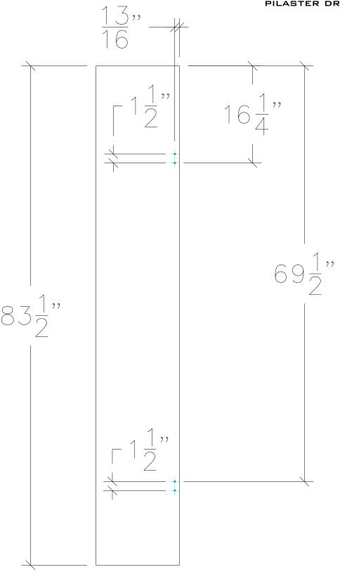
ALL HOLES SHOULD BE DRILLED WITH "F" OR 9/32" DRILL BIT
