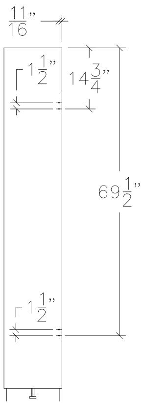
ALL HOLES SHOULD BE DRILLED WITH "F" OR 9/32" DRILL BIT
